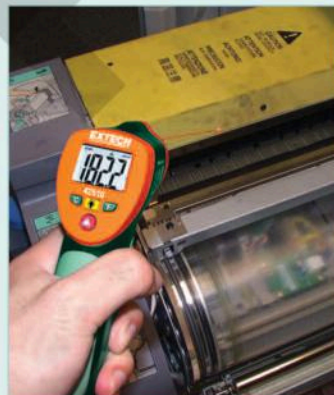
Electrical Troubleshooting for hot spot detection
